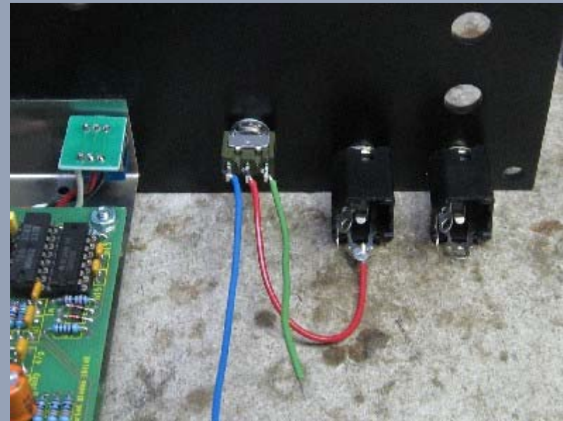
from the CHORUS (bypass) switch center lug to the MIXED OUT jack tip lug
