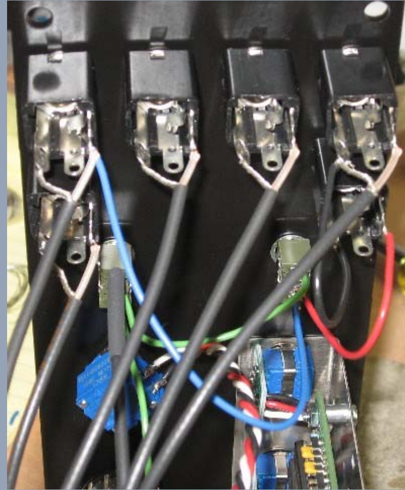
DRY (out) shield to DRY OUT jack shank lug
