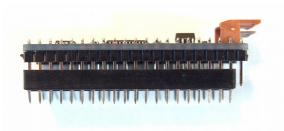
Example how to use a 20 pin strip socket to mount the CPU. Pin 1 and 42 are not connected.
