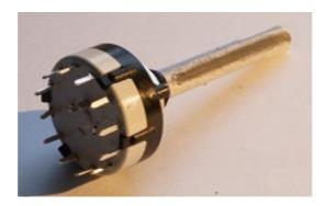
The shaft will also require cutting down. To achieve the correct length, wrap a piece of masking tape around the shaft and mark it at 25mm from the top of the bushing.
