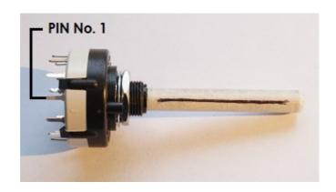
File the line away to create the flat. You don't need to file much, just enough for the cap lug screw to sit flat against and stop the cap from turning on the shaft.
