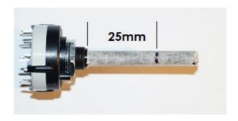
Grip the end of the shaft in a bench vice and cut with a small hacksaw.
