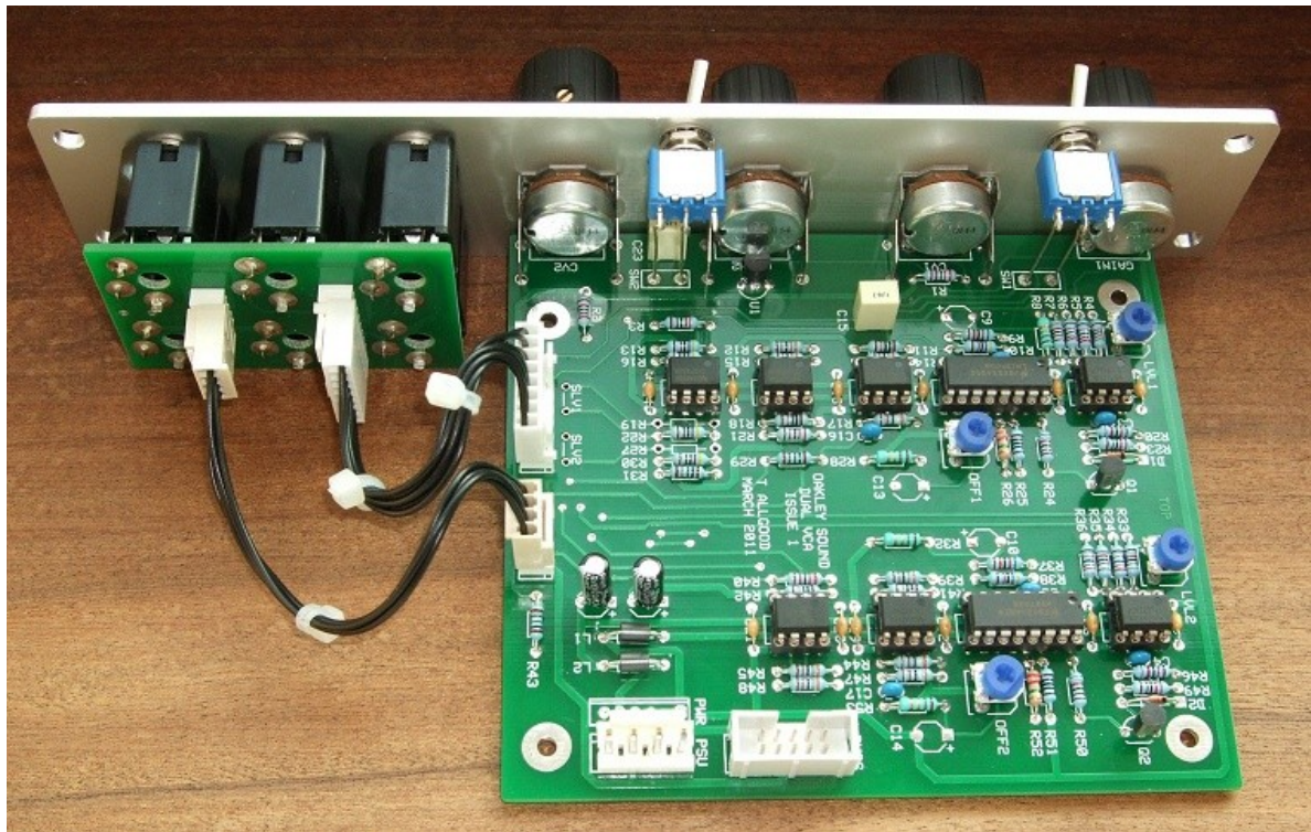
This is the original issue 1 Oakley Dual VCA module behind a natural finish 1U wide Schaeffer panel.
