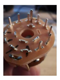
First you must clip 4 legs away for this part to fit the pcb (the ones marked with black pen). **Double check orientation before removing them**.
