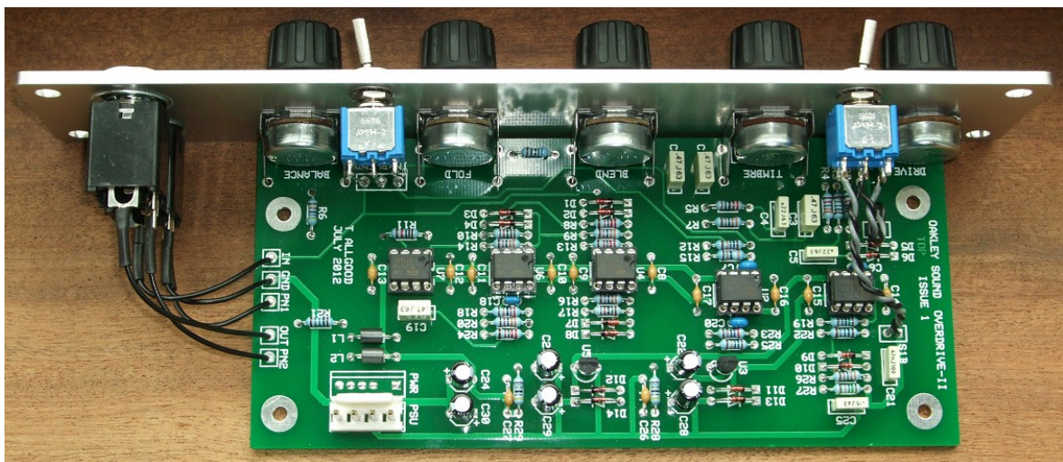
The prototype Overdrive-II fitted to a natural finish Schaeffer MOTM format panel.
