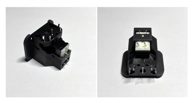
6. Solder 4 short leads to the pins of the switch, use shrink tube to protect from short-circuits with surrounding parts.
